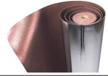
ENERGY PRO COMFORT is permanently elastic underlay made of 93% natural raw materials and polyurethane binders. ENERGY PRO COMFORT consists of a metallized PET carrier foil, a heavy-duty polyurethane layer as well as a HDPE carrier foil (in transparent). Box - 40 rolls
